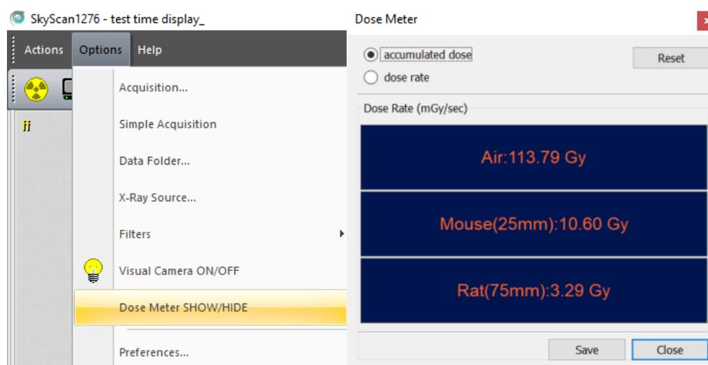
**Figure 3.** The on-screen dose meter is launched from the Options menu (left) and displays either accumulated dose or dose rate for air, mouse and rat (right).
