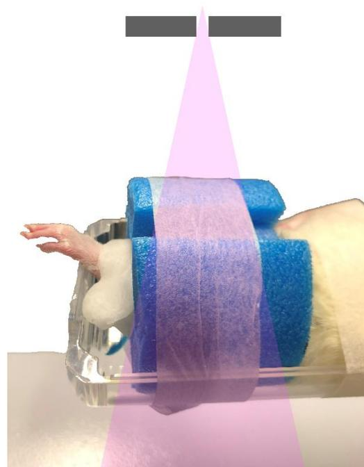
**Figure 1.** The X-ray source in the SkyScan1276 is collimated such that there is very little irradiation beyond the length (axially) of the camera field of view.
