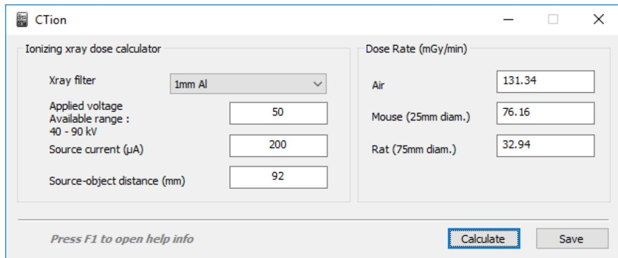
**Figure 4.** The simple window of the Bruker *CTion* X-ray dose calculator. Four inputs are needed – filter, voltage, current and object-source distance. Doses are calculated for air, mouse and rat.
