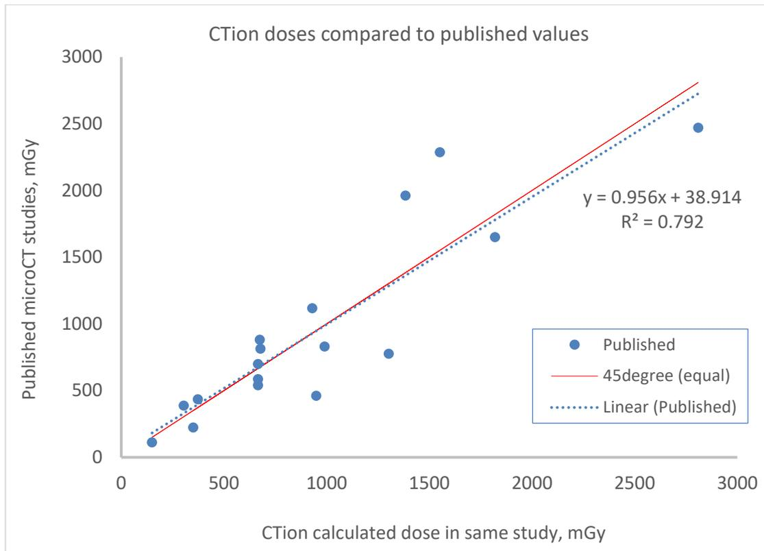
**Figure 7.** An XY plot of the data in table 4, showing published dose measurements for microCT scanners in the y axis (vertical) and corresponding dose calculation by CTion in the x axis (horizontal). The dotted blue line representing the linear regression between the published dose measurements and CTion calculations, lies close to the red line representing equality between the two.
