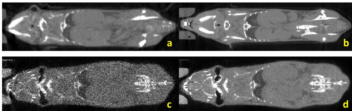
**Figure 2.** Coronal images of mouse scans, (a) by the SkyScan 1278 at 2.6 mGy and (b) at 25.8 mGy; and by a competitor scanner at 2.8 mGy (c) and at 37 mGy (d). The paired by dose comparisons of a-c and b-d show that at the same dose, the SkyScan 1278 image is of higher quality with superior signal to noise ratio.
