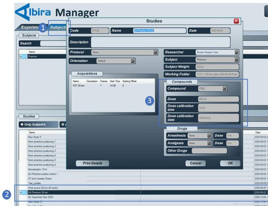
**Figure 1. Albira Software Suite NMI 3.0 Compound/Dose Registration.** To view information for an existing study 1) select the Subject and Studies Tab in the Albira Software Suite NMI 3.0 Manager view. 2) Double-click the relevant Study in the list. 3) The compound and Dose (activity in syringe at dose calibration time) is shown.
