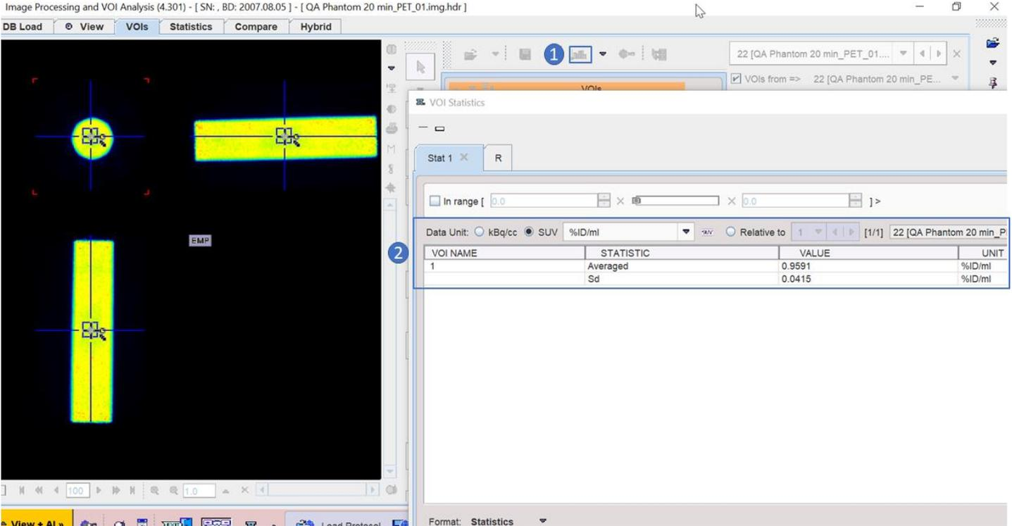
**Figure 4. %ID/mL for dynamic frames for 18F loaded cylinder phantom.** VOI is generated and 1) Statistics button is selected, 2) a Value is generated.
