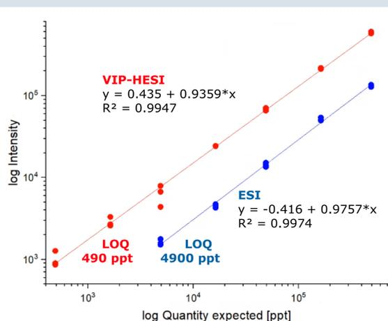
Fig. 4: Dilution series of the Lyso PE 18:1(d7) with logarithmic scaling
