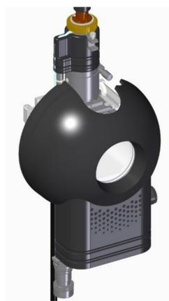
Fig. 1: Technical drawing of the VIP-HESI source
