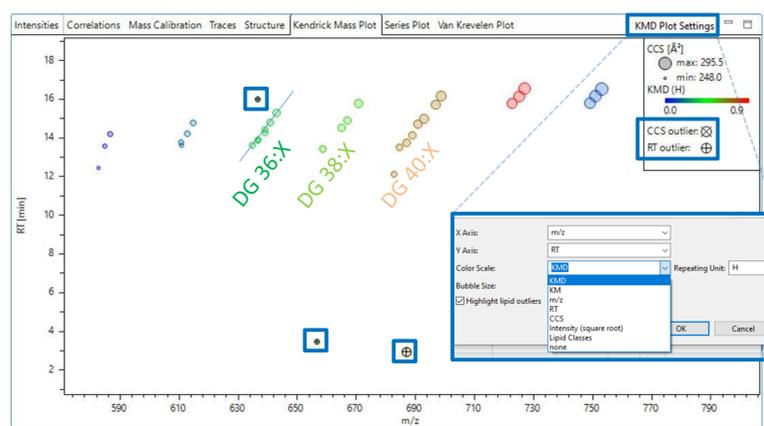
**Fig. 2: Kendrick Mass Defect Plot** filtered for DG lipids. The selected dimensions (x:  $m/z$ , y:  $R_t$ , color: KMD(H), bubble size: CCS) simplify the investigation of homologous series. The KMD(H) was plotted as color gradient to separate series of DGs with identical numbers of carbon atoms and different number of double bonds (X) in the side chains.
