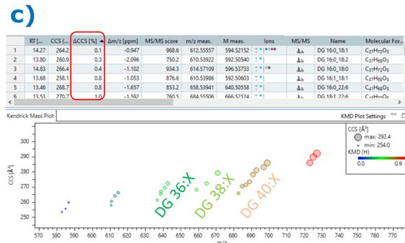
**Fig. 1a: 4D-Lipid profiling in MetaboScape.** The collisional cross section value is a physical property of an ion species in a gas phase. As such, CCS values can improve the annotation process as additional qualifiers. In MetaboScape 2022, several CCS-enabled annotation workflows can be used.
