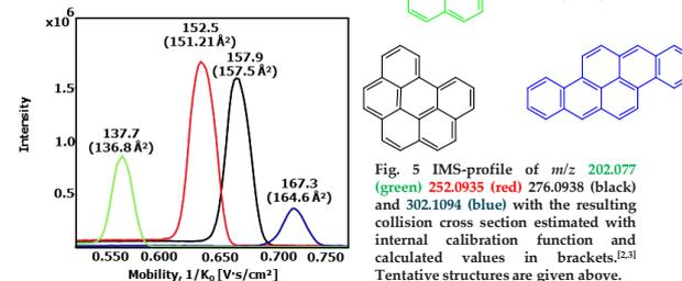
Fig. 5 IMS-profile of  $m/z$  202.077 (green) 252.0935 (red) 276.0938 (black) and 302.1094 (blue) with the resulting collision cross section estimated with internal calibration function and calculated values in brackets.<sup>[2,3]</sup> Tentative structures are given above.
