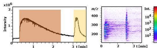
Fig. 4 a) Time-profile of the total ion current (TIC) b) Survey of the signals from diesel engine exhaust. In brown, the thermal desorption phase (250 °C) and in yellow the pyrolysis phase (450 °C) is highlighted.
