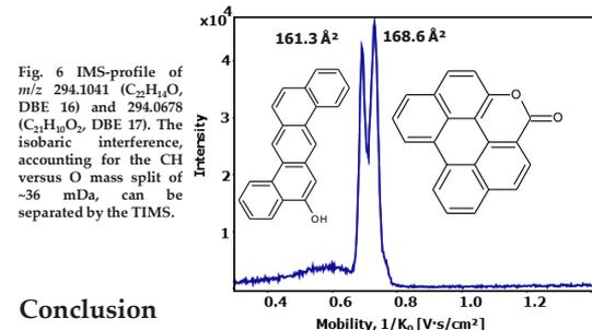
Fig. 6 IMS-profile of  $m/z$  294.1041 ( $C_{22}H_{14}O$ , DBE 16) and 294.0678 ( $C_{22}H_{10}O_2$ , DBE 17). The isobaric interference, accounting for the CH versus O mass split of ~36 mDa, can be separated by the TIMS.
