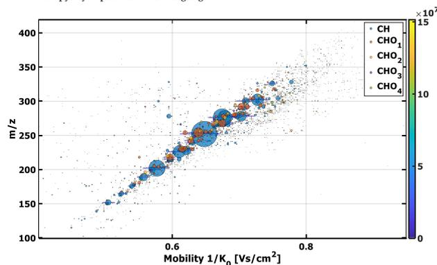
Fig. 5 Two dimensional representation of the  $m/z$  versus reduced mobility for the desorption phase of a wood combustion aerosol analyzed by DIP-APPI-TIMS-TOF. Apex peak position are given with the respective compound classes color-coded.
