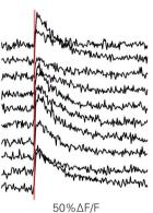
50%∆F/F 2 s Optical stimulation of selected cells containing GCaMP6s using NeuraLight 3D Ultra. Cell bodies were stimulated simultaneously by creating a 3D hologram of points with the SLM and spiral scanning all points over the cell body. Courtesy of Adam Packer, Lloyd Russell, Henry Dalgleish, and Michael Hausser (University College London).
