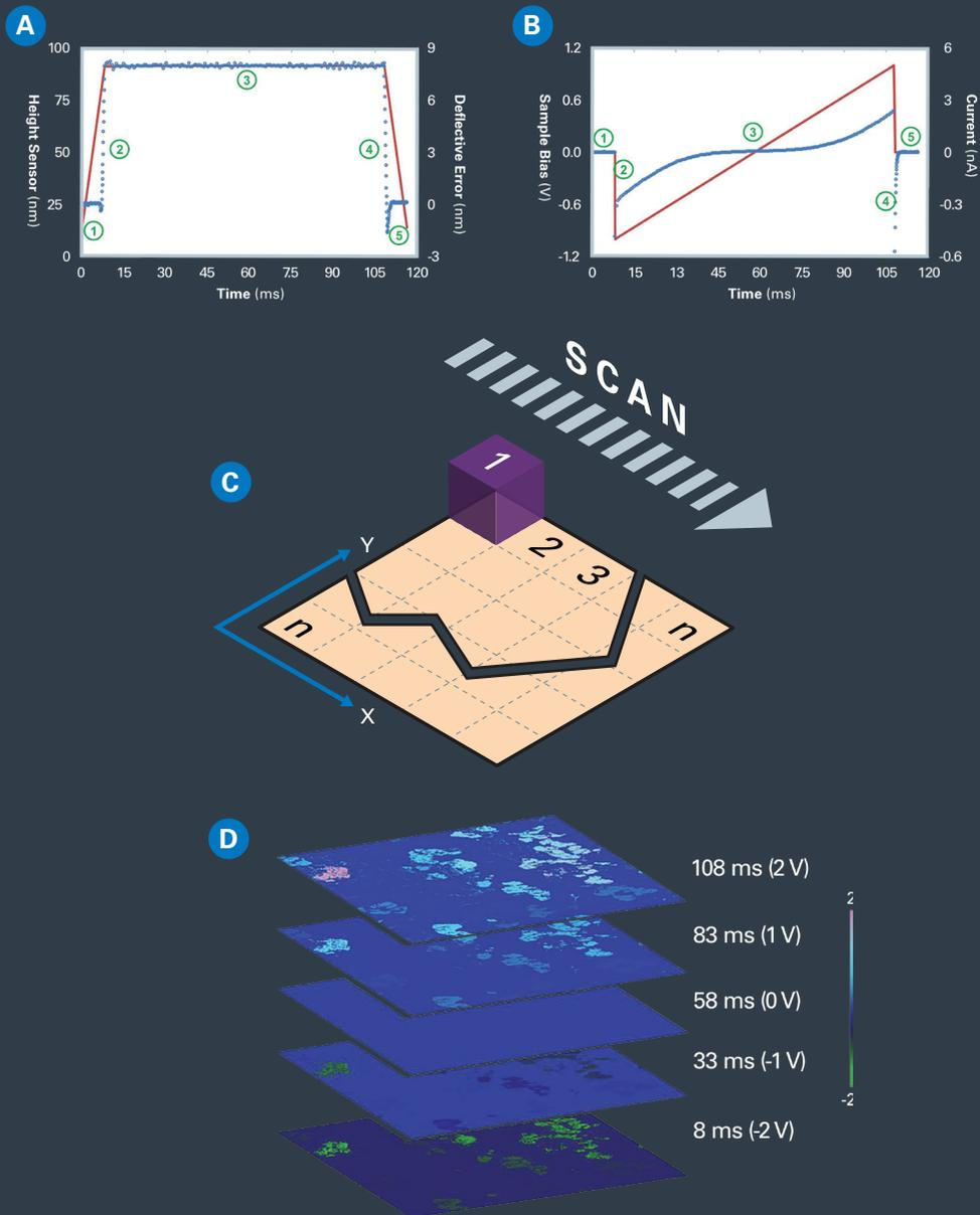
This avoids the shear force that is common in contact mode-based scanning. Section (D) of the figure shows five typical current slices extracted from a data cube acquired using this principle on  $\gamma\text{-Fe}_2\text{O}_3$ .
