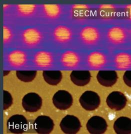
(from top) Three data channels from donut-shaped thiol self-assembled monolayer on Au,  $\text{Si}_3\text{N}_4$  layer with openings on Pt. Scan sizes (X): 25  $\mu\text{m}$ , 5  $\mu\text{m}$ .
