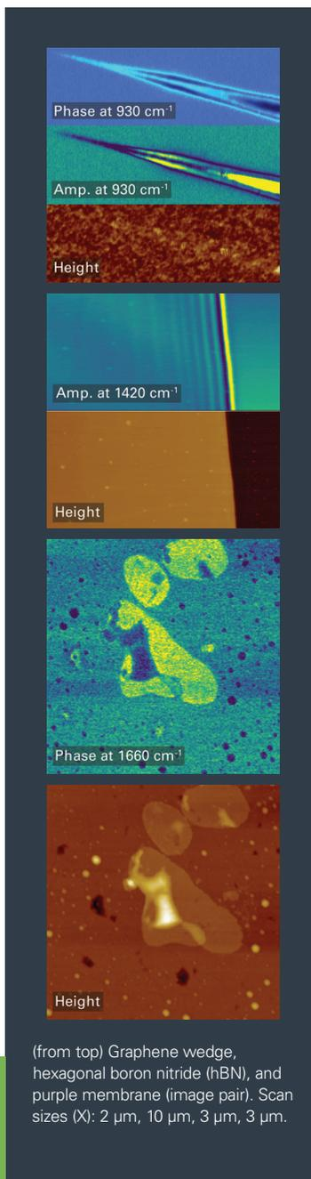
(from top) Graphene wedge, hexagonal boron nitride (hBN), and purple membrane (image pair). Scan sizes (X): 2  $\mu\text{m}$ , 10  $\mu\text{m}$ , 3  $\mu\text{m}$ , 3  $\mu\text{m}$ .
