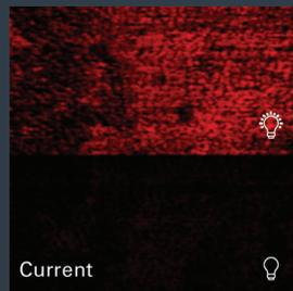
(from top, in pairs) Illuminated composite CNT/P3HT sample and P3HT/PCBM sample illuminated and dark without bias. Scan sizes (X): 700 nm, 1  $\mu$ m. (courtesy Dr. Philippe Leclère, University of Mons, Belgium)
