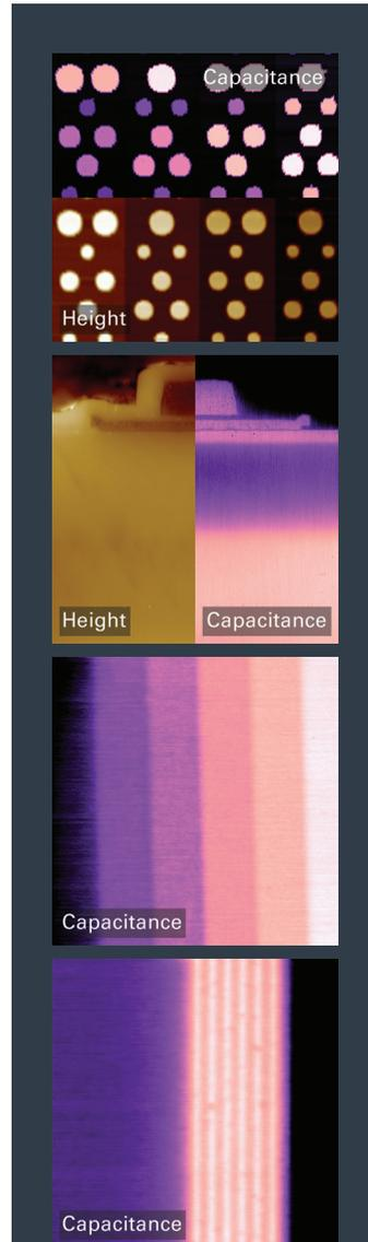
(from top) Array of small capacitors, and carrier profiling on cross-section of PIN diode, Si sample with staircase dopant profile, and sample with alternating doped Si/SiO<sub>2</sub> layers. Scan sizes (X): 46  $\mu\text{m}$ , 25  $\mu\text{m}$ , 13  $\mu\text{m}$ , 2  $\mu\text{m}$ .
