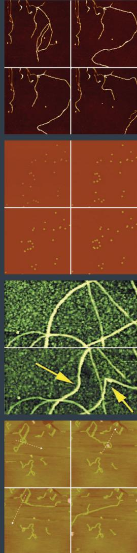
Height images during manipulation of (from top) carbon nanotubes, Au nanoparticles, carbon nanotubes, and polymer macromolecule on HOPG. Scan sizes (X): 2  $\mu\text{m}$ , 2  $\mu\text{m}$ , 900 nm, 500 nm.
