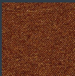
Height images of (from top) dinoadecanoylbenzene, monolayer at the phenyloctane/HOPG interface, selenol-based aromatic SAM, and HOPG atoms. Scan sizes (X): 15 nm, 20 nm, 10 nm, 12 nm.
