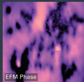
(from top) Thermoplastic vulcanizate with low modulus EPDM, harder polypropylene, and (charged) carbon black nanoparticles. Scan sizes (X): 3  $\mu\text{m}$ , 3  $\mu\text{m}$ , 3  $\mu\text{m}$ .
