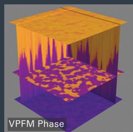
(from top) Thin films of BFO (after domain manipulation), PMN-PT, and LTO. (bottom) DataCube PFM Phase switching displayed vs. applied voltage on a BFO film. Scan sizes (X): 5  $\mu\text{m}$ , 10  $\mu\text{m}$ , 1  $\mu\text{m}$ , 1  $\mu\text{m}$ .
