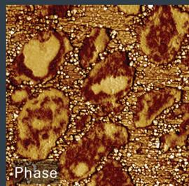
(from top, in pairs) Impact-modified copolymer and rubber. Scan sizes (X): 8 μm, 4 μm.
