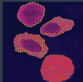
(from top, all MFM phase) Nickel alloy, Permalloy, Co-Pd multilayers showing clear domain structures, and magnetic heterostructures (Courtesy: AG Hellwig, TU Chemnitz). Scan sizes (X): 13  $\mu\text{m}$ , 30  $\mu\text{m}$ , 9  $\mu\text{m}$ .
