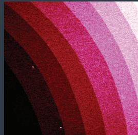
Height images of (from top) epitaxial Si, 100 nm polystyrene spheres, diatom in marine gel, and atomic step terraces. Scan sizes (X): 1  $\mu\text{m}$ , 6  $\mu\text{m}$ , 5  $\mu\text{m}$ , 5  $\mu\text{m}$ .
