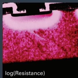
(from top) Cross-sectioned battery cathode, and carrier concentration maps in cross-sectioned Si transistor and Si DPMOSFET device. Scan sizes (X): 15  $\mu\text{m}$ , 6  $\mu\text{m}$ , 12  $\mu\text{m}$ .
