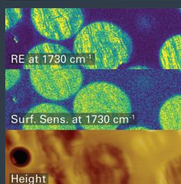
(from top) Thin PS film on thick acrylate with accompanying IR spectra, PMMA wedge on Si, PMMA in epoxy. Scan sizes (X): 5  $\mu\text{m}$ , 2.4  $\mu\text{m}$ , 10  $\mu\text{m}$ .
