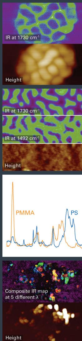
(from top) Block copolymer core shell, PMMA/PS block copolymer with accompanying IR spectra, and nanocontaminants on a wafer. Scan sizes (X): 400 nm, 500 nm, 2  $\mu\text{m}$ .
