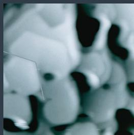
(from top, all in-situ height) SEI failures in Li-ion batteries through lithation/delithiation, Cu deposition on glassy carbon, deposited Fe nanoparticles, and overpotential deposition of Cd on Cu(111). Scan sizes (X): 5  $\mu\text{m}$ , 1  $\mu\text{m}$ , 2  $\mu\text{m}$ , 650 nm.
