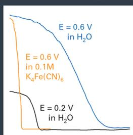
Height images of (from top) HOPG in water, Sn<sub>80</sub>Pb<sub>40</sub> in glycerol, and Cd-Ni coating. (bottom) Potential-distance profiles across electric double layers. Scan sizes (X): 10 nm, 5  $\mu$ m, 10  $\mu$ m.
