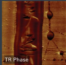
(from top, in pairs) HOPG with water at the step edges and PDES on Si substrate showing anisotropic property data in the TR phase channel. Scan sizes (X): 3  $\mu\text{m}$ , 12  $\mu\text{m}$ .
