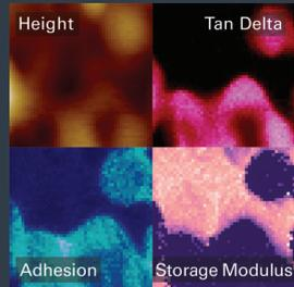
(from top) Quaternary polymer blend with correlated rheological frequency spectra, PEE, and PC-ABS polymers. Scan sizes (X): 8  $\mu\text{m}$ , 1.5  $\mu\text{m}$ , 1  $\mu\text{m}$ .
