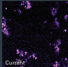
(from top, in pairs) Rubber modified PP with carbon nanoparticles and carbon sticky tape with conductive carbon nanoparticles. Scan sizes (X): 4  $\mu\text{m}$ , 5  $\mu\text{m}$ .
