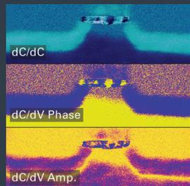
(from top) SCM carrier profile images on Si CCD sensor, Si SRAM memory, two adjacent transistors (top surface), and a cross-sectioned PMOS transistor. Scan sizes (X): 10  $\mu\text{m}$ , 22  $\mu\text{m}$ , 1  $\mu\text{m}$ , 600 nm.
