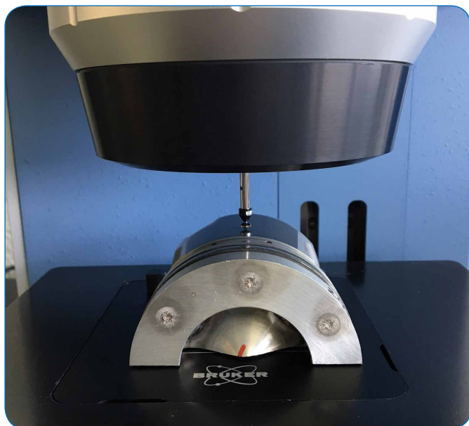
Figure 1: Halved piston from a diesel combustion engine.
