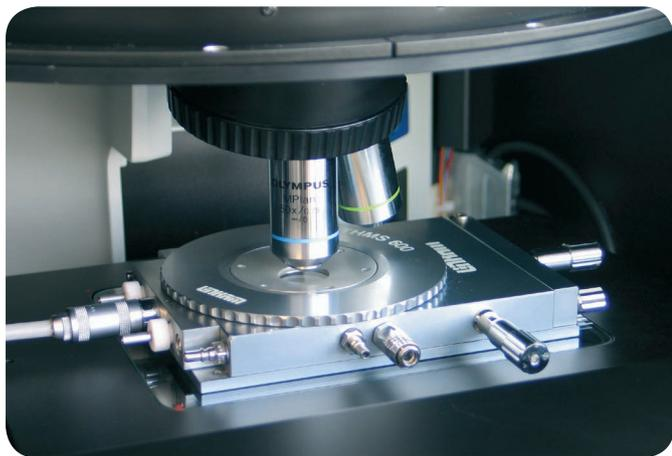
Abb. 4 Linkam stage in the sample compartment of the SENTERRA II<sup>(4)</sup>
