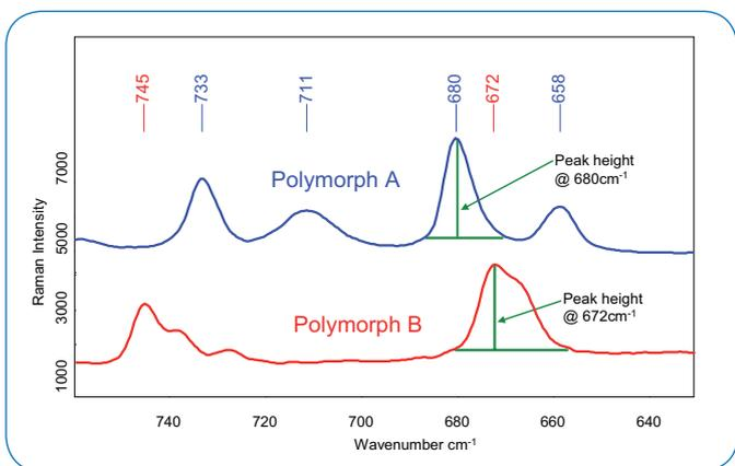
Fig. 5 Raman spectra of polymorph A and B; relevant spectral region
