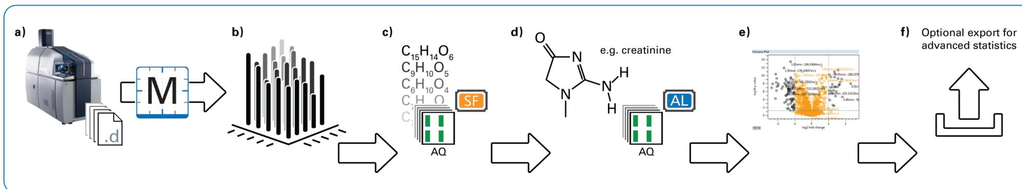
Fig. 1: Schematic (1) MRMS aXelerate workflow: a) FIA-MRMS acquisition using a scimaX MRMS, b) Data processing and evaluation using T-ReX 2D in MetaboScape 4.0, c) Generate list of molecular formula annotations including annotation qualities, d) Putative metabolite annotations using AnalyteList of known and expected compounds, e) Statistical analysis to identify features of interest, f) Optional export for advanced statistical analyses.
