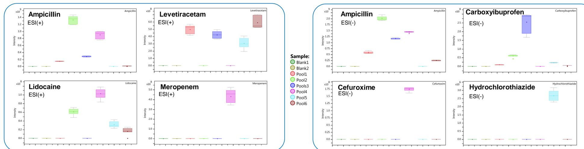
Fig. 2a: Bucket statistic (box plots) of tentatively annotated drugs in pooled urine samples using FIA-MRMS in positive ion mode.
