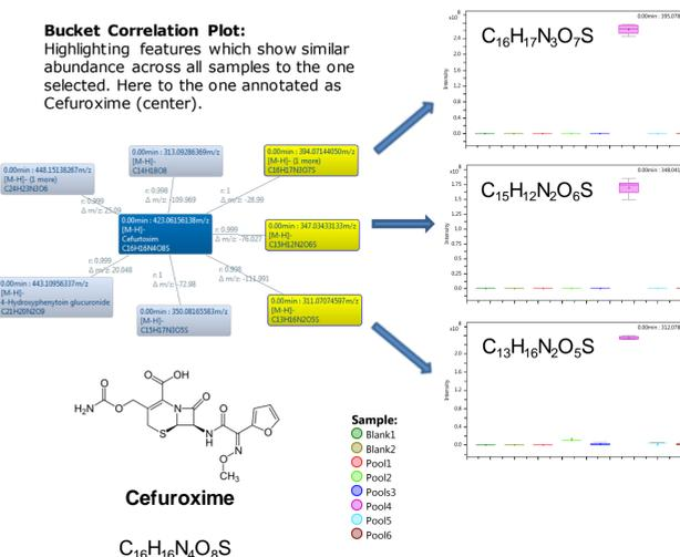
Fig. 3: Detection of possible metabolites of Cefuroxime in ESI(-) using Bucket Correlation Plot (left). Feature can be directly annotated with molecular formula due to very accurate mass detection.
