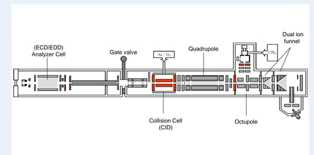
**Figure 2.** Diagram of the 12T Bruker solarix XR FT-ICR MS
