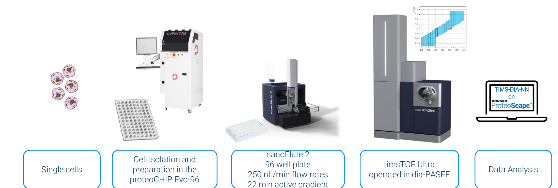
Figure 7: Single cell proteomics workflow with proteoCHIP Evo-96 transfer to 96 well plates, injection with nanoElute 2 on the timsTOF Ultra.
