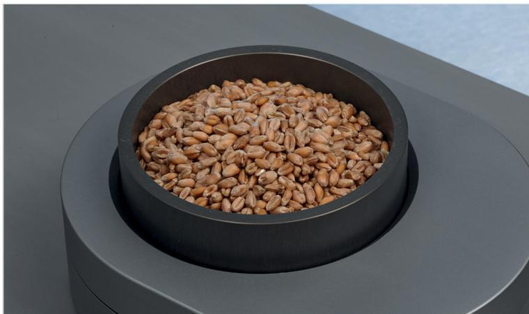
Analysis of solid products (here unground wheat) on the integrating sphere of the TANGO-R in diffuse reflection. Cereal grains can be measured in a ground or unground state, depending on the analysis requirements.
