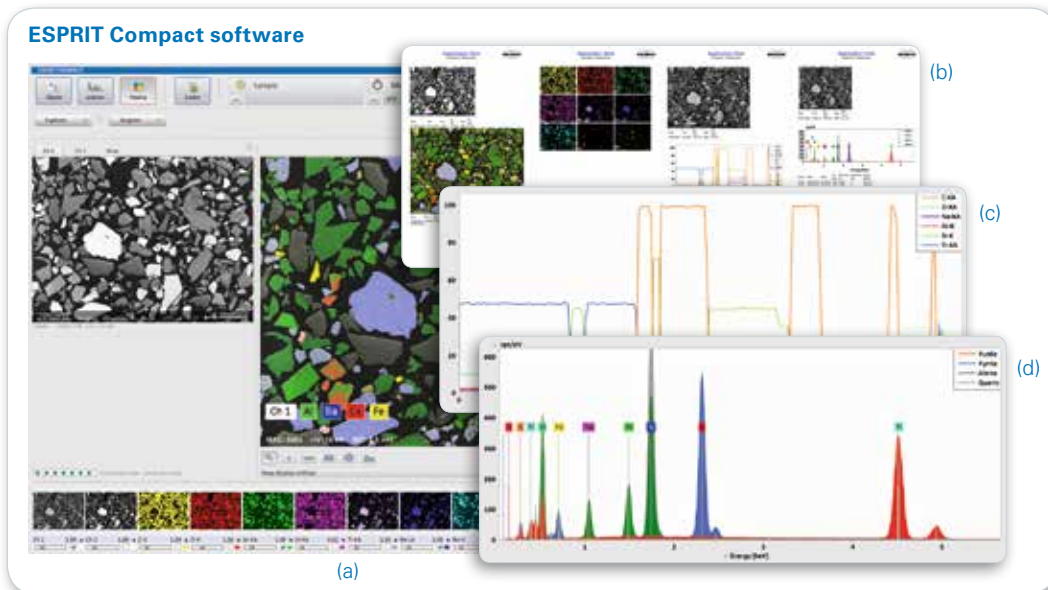
ESPRIT Compact with mapping (a), report (b), line scan (c), and spectrum (d)
