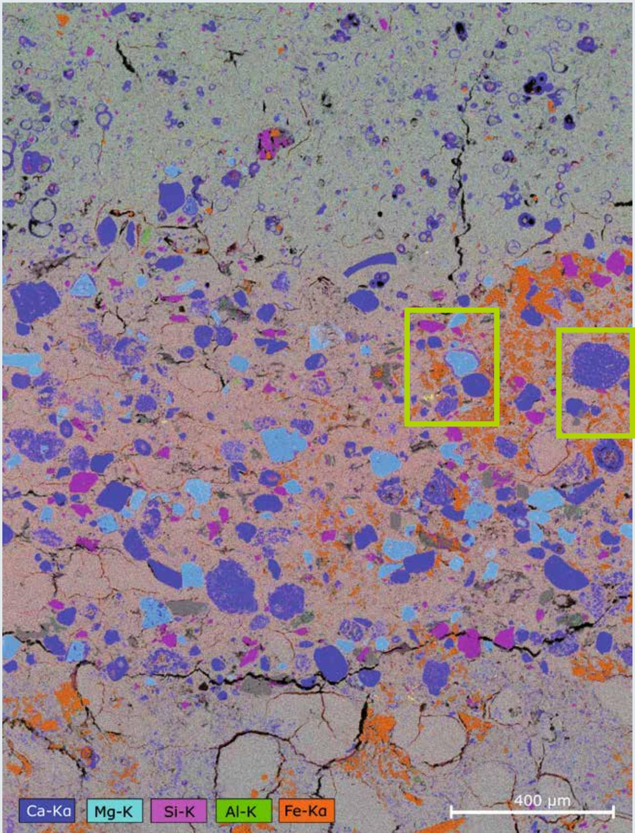
Fig. 1 High resolution EDS map (3072 x 4096 pixels) showing the uppermost part of the ejecta deposit in ODP Leg 207 and the transition to the early Palaeogene claystone above. Note that the occurrence of carbonates (calcite, dolomite) and quartz is clearly restricted to the top 0.5 to 0.7 mm of the ejecta deposit. The areas in the green rectangles were magnified in Fig. 3.
