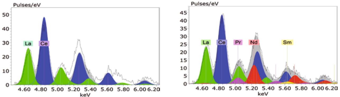
Fig. 4 Deconvolution of overlapped, background corrected peaks without (left) and with (right) consideration of praseodymium and samarium. Each color represents the deconvoluted peak for one element; the grey peak in the background is the sum of the deconvoluted peaks. The black line is the measured spectrum.
