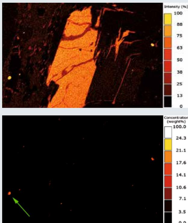
Fig. 3 Comparison of the element distribution of cerium. Top: ROI map showing intensity of Ce-L $\alpha$  (%). Bottom: background corrected QMap showing Ce concentration (weight %); the arrow points to the phase containing cerium (see Tab. 1).
