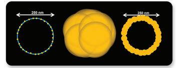
Figure 1. Single-molecule localization principles. Example of the sample to be imaged in a diffraction limited volume (left), image of the diffraction limited volume with traditional microscopy methods (middle), image of diffraction limited volume with SMLM (right).
