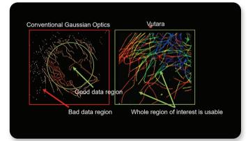
Figure 3. Vutara's top-hat illumination technology. By illuminating the entire field of view, the Vutara enables quality imaging for the entire plane, resulting in acquisitions suitable for quantitative analysis.
