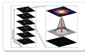
Figure 2. Image acquisitions of single molecules over time with SMLM. Each molecule is imaged stochastically within an imaging plane over time. The point spread function data are collected and used to localize the center of each individual molecule.
