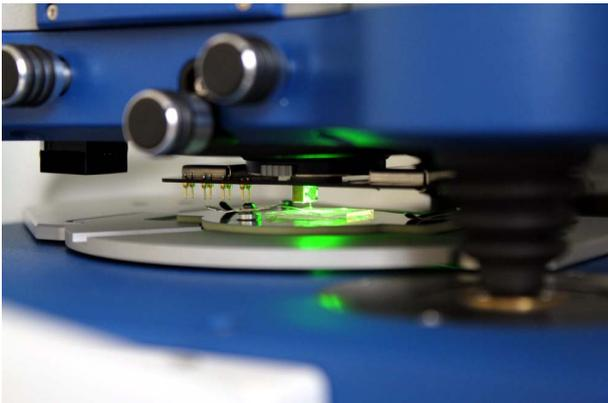
*Combined STM and optics: NanoWizard® 3 equipped with STM-Module on Zeiss inverted optical microscope*
