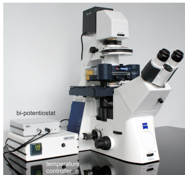
Figure 2: SECM option on NanoWizard 4 XP on a Zeiss Axio-Observer inverted optical microscope
