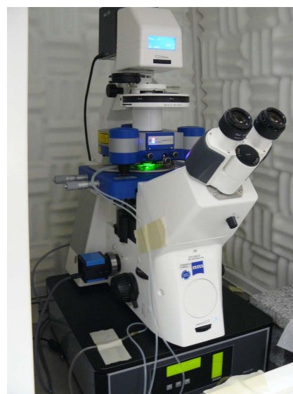
Fig. 2: Experimental setup used for the investigations. The NanoWizard® AFM with the mounted conductive module is integrated into an inverted microscope (Zeiss, AxioObserver), which rests on an active vibration platform (Accurion, micro 40). The tubes are connecting the closed chamber CAFM module with a nitrogen source. The microscope is equipped with transmission illumination (condenser), fluorescence illumination and a CCD camera.
