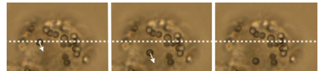
Fig. 3: Manipulation of particles inside living cells. Macrophages readily engulf particles presented to their surface. These internalized particles can be manipulated with optical traps as indicated by the white arrow. The dashed line marks the initial position of the bead.
