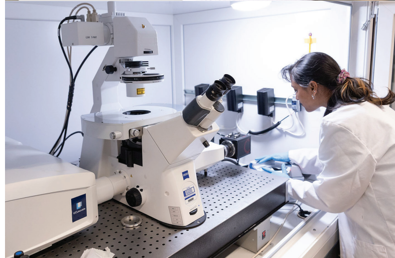
BioAFM is an important tool in Dr. Alsteens's lab for imaging and analyzing proteins, receptors, viruses, and cells at the single-molecule level.
