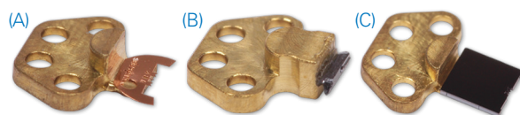
Figure 3. (A) Bulk sample mount, (B) Si wedge sample mount, and (C) PTP sample mount for advanced front end.
