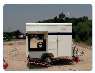
Atmosfir Optics Ltd. and Bruker Optics have come together to provide a complete, fully automated, and reliable fence-line monitoring system. Combining Bruker's Open Path FT-IR technology with Atmosfir's data analysis and management algorithms yields the world's most versatile, sensitive, and cost-effective fence-line technology: the D-fenceline<sup>TM</sup> monitoring and air quality management system.
