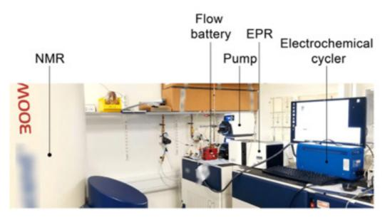
Figure 2: Online EPR-NMR set up for studying of Organic RFB's. Involved is an electrochemical cycler, two peristaltic pumps, RFB, benchtop Magnettech ESR5000 EPR (Bruker), and 300 MHz NMR (Bruker).<sup>1</sup>
