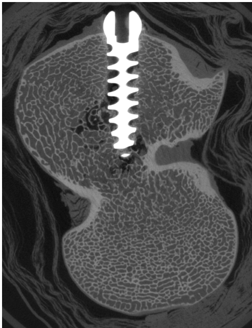
Figure 2: Section through a titanium screw in the condyle of a sheep femur; minimal density artefacts allow visualisation of undamaged trabeculae between the screw blades.
