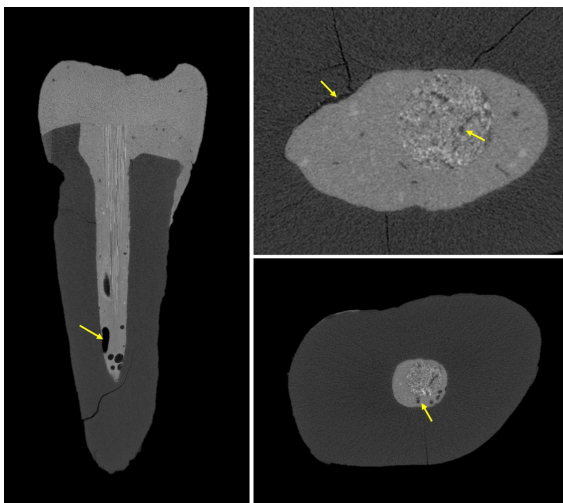
Figure 1: Reconstructed slices visualizing gaps between the cavity restoration and access cavity walls, and voids within the cavity restoration, 4 \mu m isotropic voxel size
