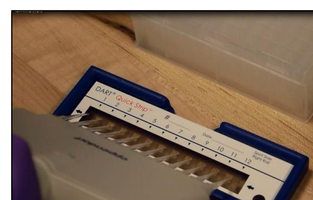
Figure 1: QuickStrip™ module on automated presentation robotics with JumpShot equipped DART-MS
