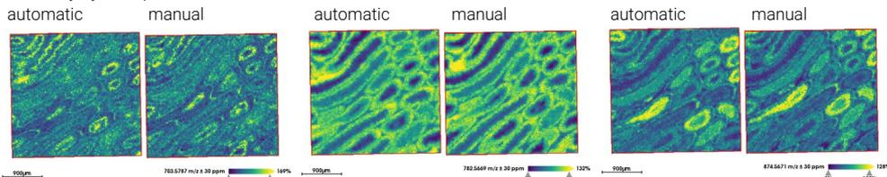
Representative ion images of a rat testis dataset measured on the timsTOF fleX in the lipid range with 20 μm pixel size using either the automatic or the manual workflow to set-up the acquisition. The ion intensities and distributions are similar in both cases.
