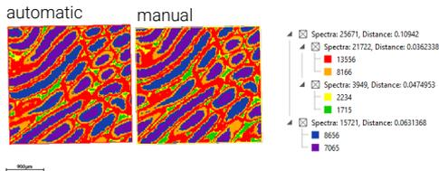
Segmentation map of the lipid imaging dataset after automatic and manual acquisition set-up demonstrating that the tissue type is the main discriminating factor rather than the acquisition set-up method.
