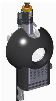
Fig. 1: Technical drawing of the VIP-HESI source
