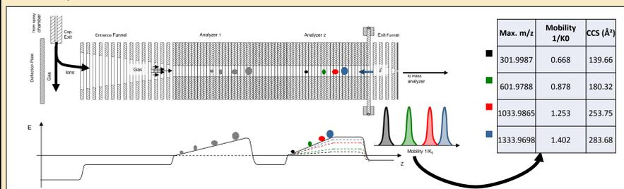
Fig. 2. (Above) Ions exit the capillary and enter the first funnel, then trapped in analyzer 1. Ions are transferred to analyzer 2 where they are separated further, and elute separately to the mass analyzer.
