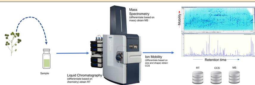
Fig. 1. General UHPLC-TIMS-MS/MS metabolomics workflow. Sample is prepared, LC, TIMS, and MS data are acquired. Data is then compared with reference databases.
