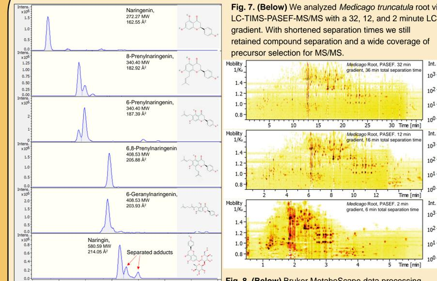
Fig. 7. (Below) We analyzed *Medicago truncatula* root via LC-TIMS-PASEF-MS/MS with a 32, 12, and 2 minute LC gradient. With shortened separation times we still retained compound separation and a wide coverage of precursor selection for MS/MS.
