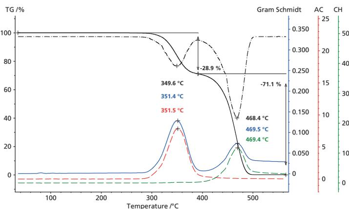
To identify the decomposition products, 2-D spectra can be extracted from the 3-D cube shown above and subjected to a library search. In the present case, analysis of the FT-IR absorption intensities shows the release of acetic acid and various hydrocarbons.
