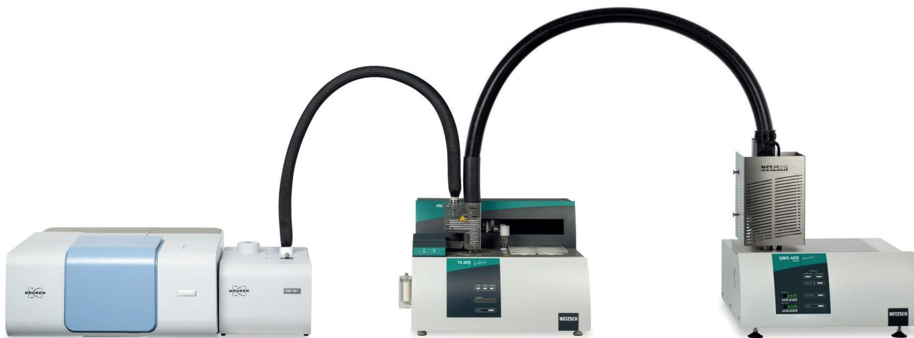
All NETZSCH thermobalances (TGAs) and simultaneous thermal analyzers (STAs) are characterized by their vertical, top-loading design. This not only guarantees easy operation and sample loading, but is also in accordance with the natural gas flow path inside the furnace (warm gases have the tendency to rise) and protects the balance in an optimal way.
