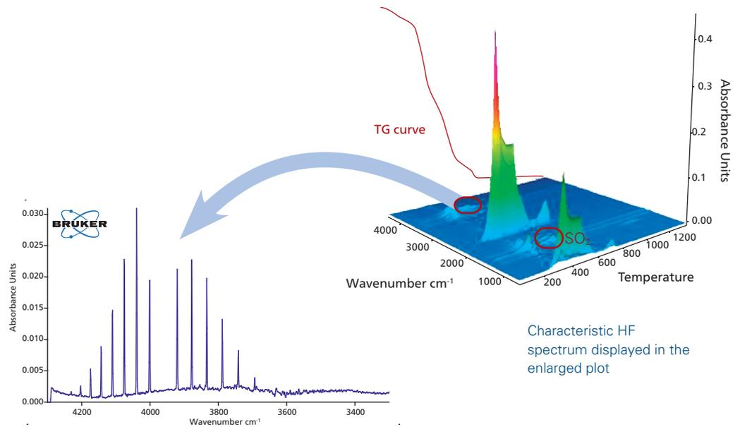
Characteristic HF spectrum displayed in the enlarged plot
