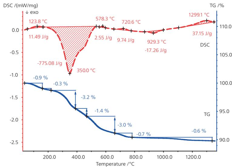
Mass changes and energetic changes of a clay for porous bricks; presentation of the TGAS curve (blue) and the corresponding DSC curve (red).
