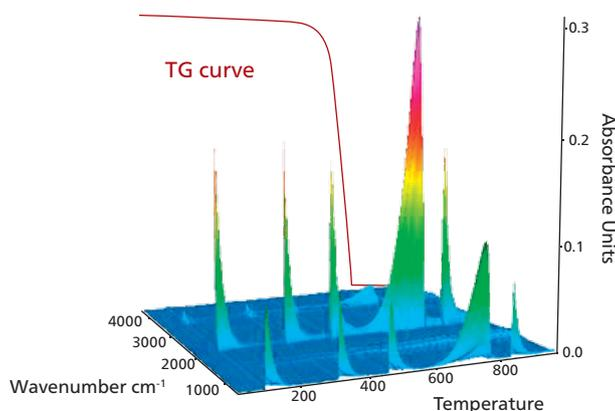
3-D plot for CO<sub>2</sub> calibration pulses and CaCO<sub>3</sub> decomposition; pulses for quantification need to be repeatable and temperature-independent (a linear relationship to the injected gas concentration)
