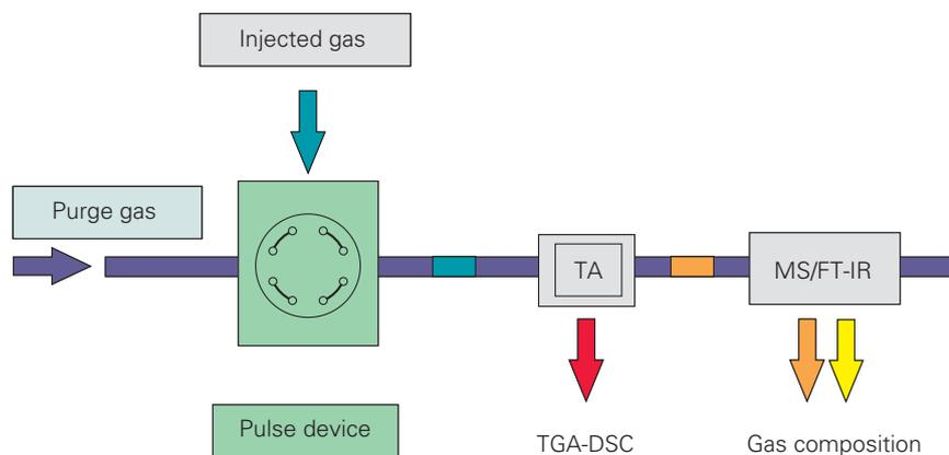
PulseTA<sup>®</sup> allows for three types of thermoanalytical experiments:
