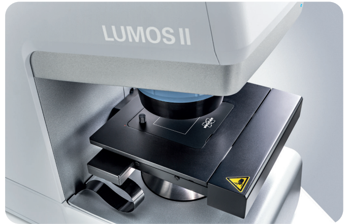
Figure 3: Sample on the stage of the LUMOS II FT-IR microscope.
