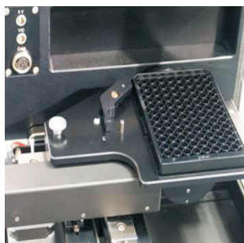
Fig. 4 HTS-Raman accessory mounted in the FT-Raman sample compartment
