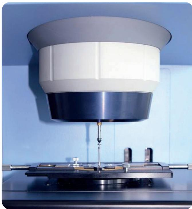
Figure 1: Needle mounted in a sample holder vise.
