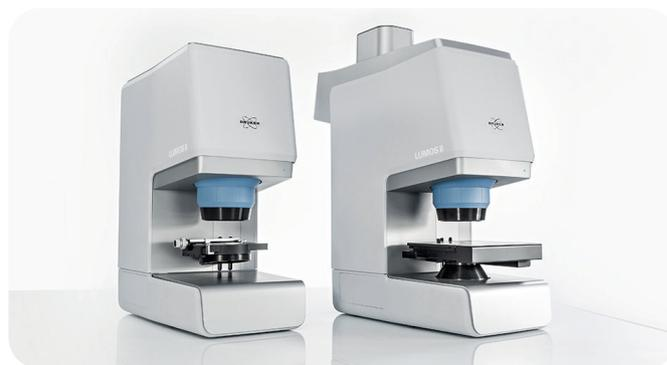
The FT-IR microscope LUMOS II replaced its predecessor in 2019 and now also offers FPA imaging technology. The measurements in this application note were performed with a LUMOS, but are **of course** also feasible with the LUMOS II.
