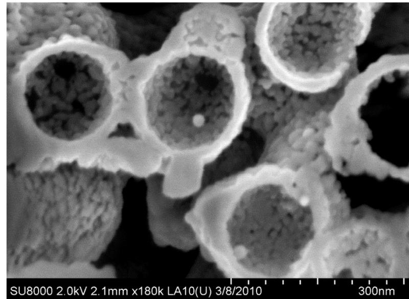
Porous Zirconium shell with active catalyst particle
