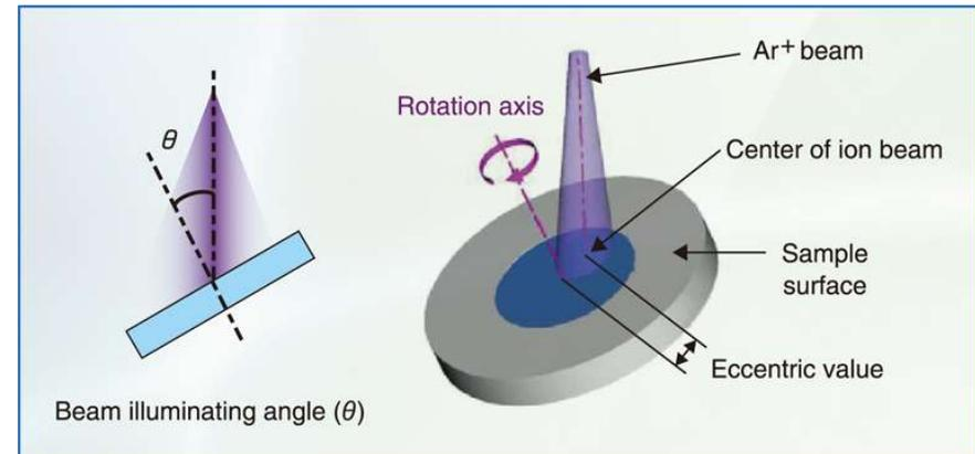
Flat milling method: Shifts the beam over the surface to uniformly sputter-etch the sample with Argon ions
