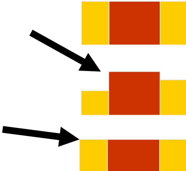
Angles  $>15^\circ \Rightarrow$  Selective etching (chemistry, orientation)
