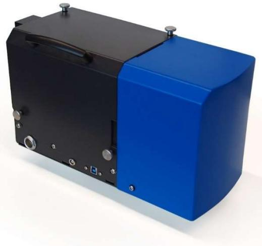
Compact CL system for high-performance (RGB) intensity CL mapping
