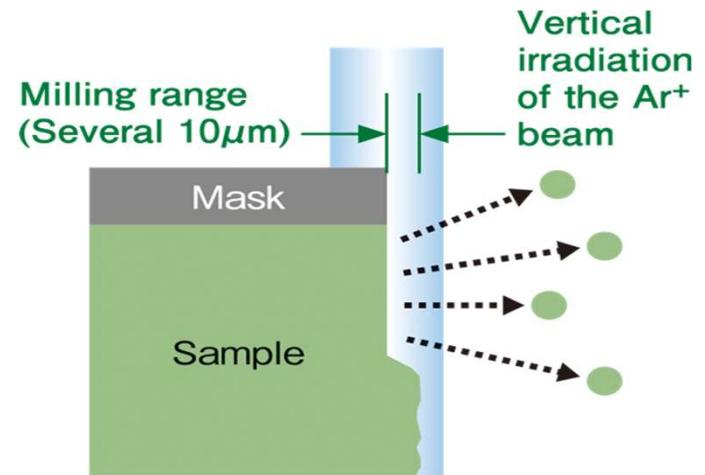
Cross-section Milling: Sputter-etch the sample with Ar ions partly covered with a mask to gradually produce a sharp edge
