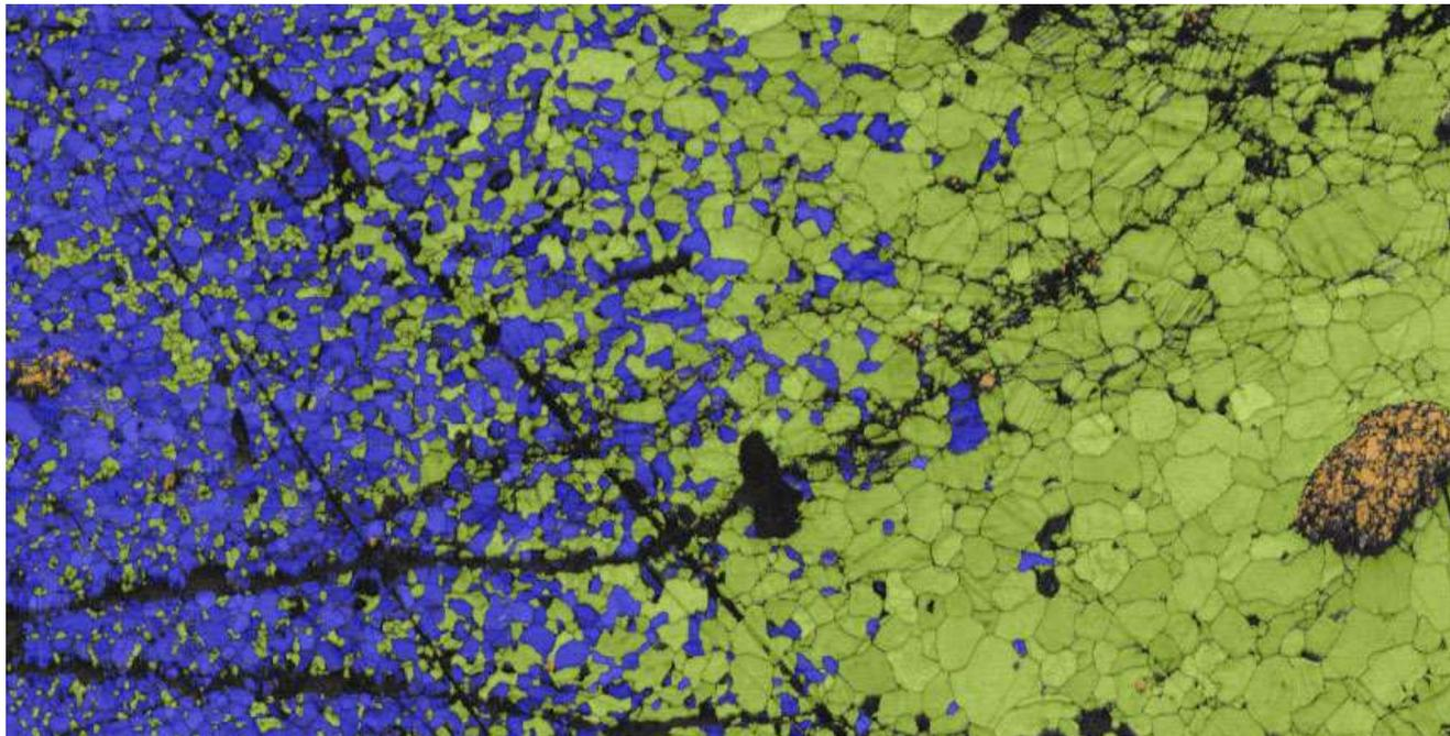
EBSD can distinguish chemically identical phases such as calcite and aragonite
