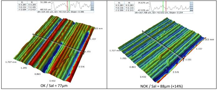
Figure 1: 3D morphology Comparison of 3D printed PEEK lab-on chip components Parts Courtesy Denis Dowling, University College Dublin
