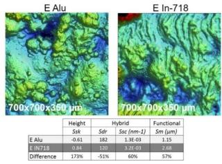
Figure 2: 3D surface morphology of comparison between Aluminium and Inconel manufactured rings
