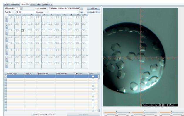
Figure 2: ISX stage control software with plate navigation area, image viewer, and job queue.
