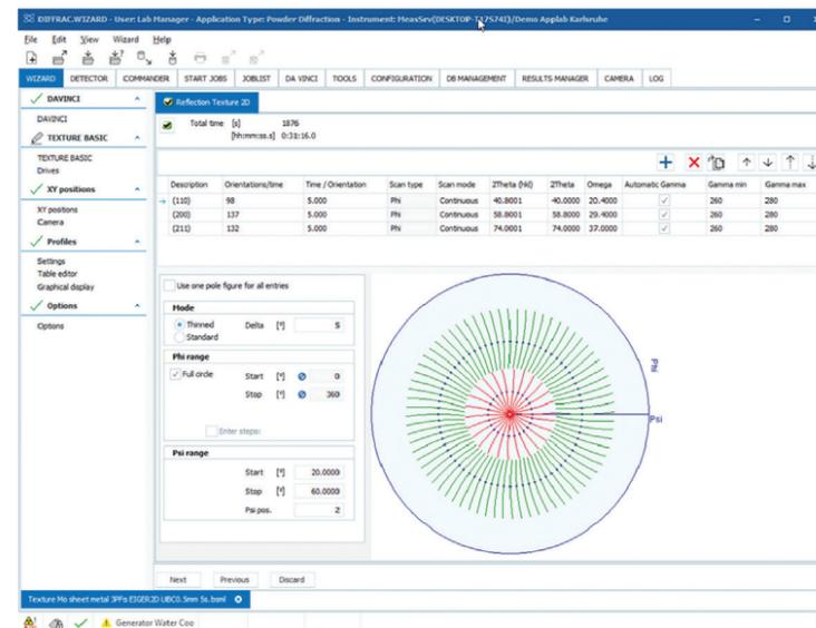
**Fig. 2** Pole figure measurement planning in DIFFRACT.WIZARD.
