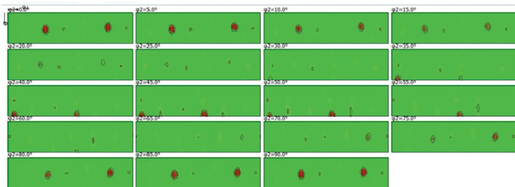
**Fig. 5** Orientation distribution function (ODF) for the molybdenum sheet metal.
