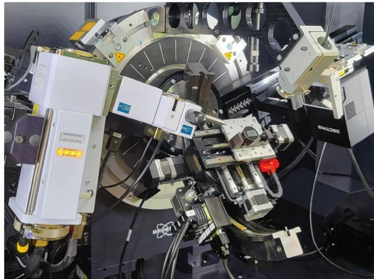
**Fig. 1** D8 DISCOVER configured for the measurement of pole figures.
