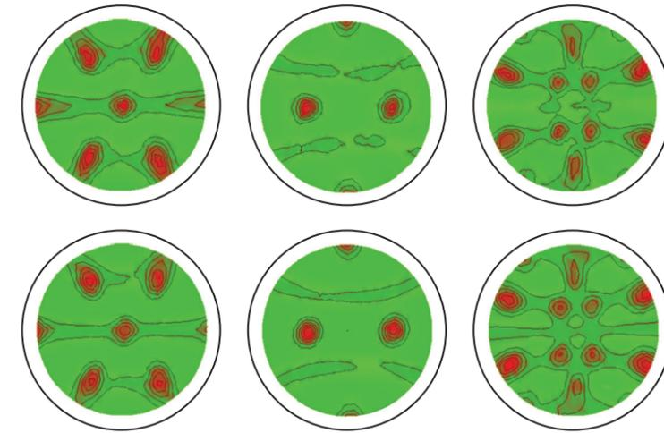
**Fig. 3** Experimental (top) and recalculated (bottom) (110), (200) and (211) pole figures of the molybdenum sheet metal.
