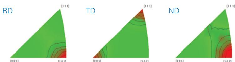
**Fig. 6** Inverse pole figure (IPF) obtained for the molybdenum sheet metal.
