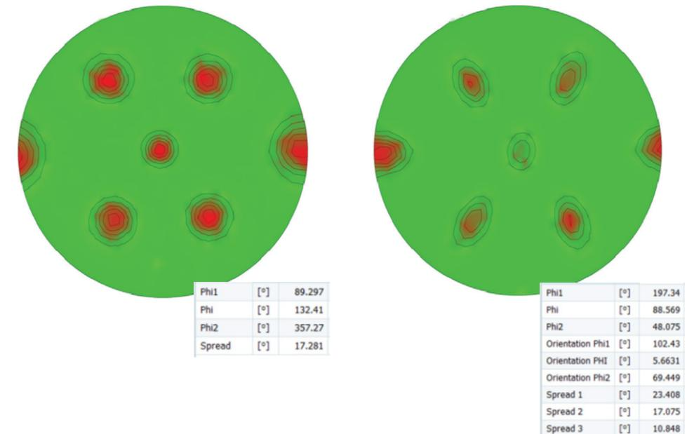
**Fig. 4** Recalculated (110) pole figure using a single spherical (left) and elliptical (right) component. The table shows the additional degrees of freedom allowed for elliptical components.
