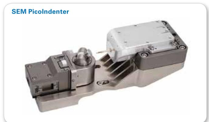
Fig. 1 Bruker's Hysitron PI 88 SEM PicoIndenter
