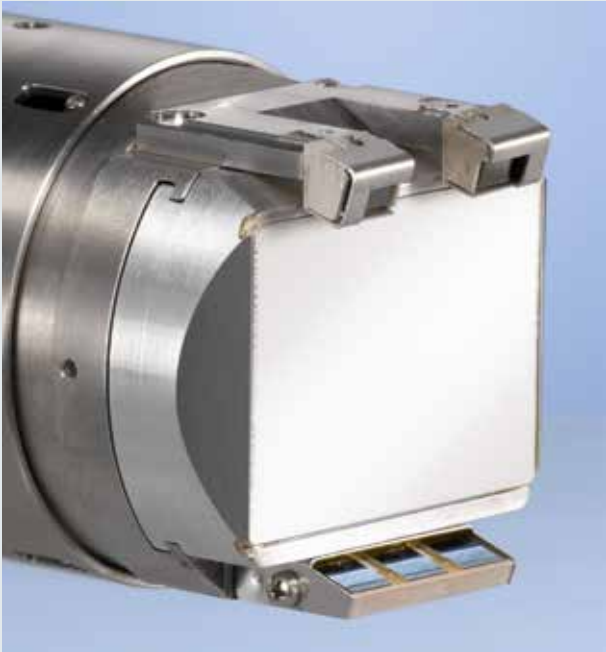
Fig. 1: Left – ARGUS™ FSE/BSE detectors and phosphor screen; right top – tensile stage inside the SEM chamber as seen from the EBSD port; right bottom – drawing of sample dimensions (values are given in mm).
