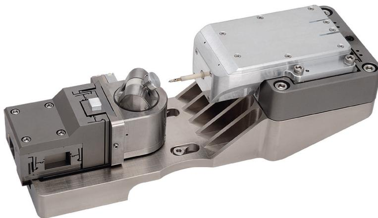
When equipped with the optional tilt and rotation stages, the PI 88 SEM PicoIndenter features flexible sample positioning with five degrees of freedom (X, Y, Z, tilt, rotation) giving the user the ability to align the sample with an ion beam for sample preparation or with detectors such as EBSD, EDS, or WDS to obtain a deeper understanding of the material's mechanical response.
