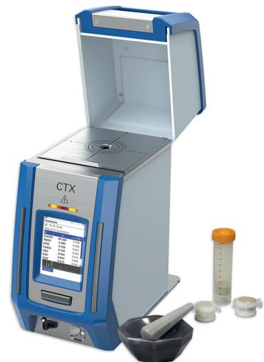
and the start trigger is pressed. Measurement results begin appearing on the screen immediately. The measurement precision can be tested with repeated measurements using a known catalytic converter powder sample. Homogeneity of the powder can be tested by performing multiple measurements. To take into account possible sample variability, it is also important to take multiple samples from the material batch and use the averaging feature.
