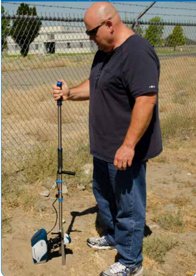
GPS integration for geospatial mapping and smart XRF sampling of large areas
