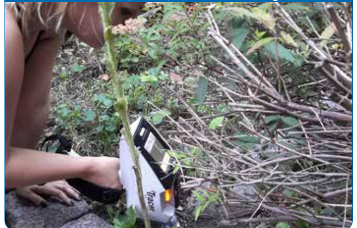
Handheld XRF (HHXRF) is ideal for screening soils
