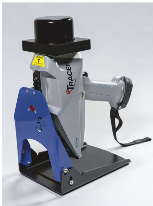
Figure 2 TRACER 5 desktop stand kit with safety shield in place
