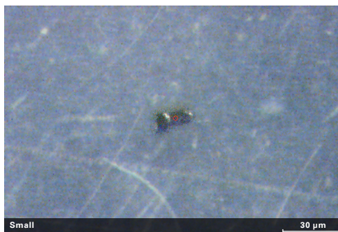
Figure 4 Inclusion of a small particle in a plastic film
