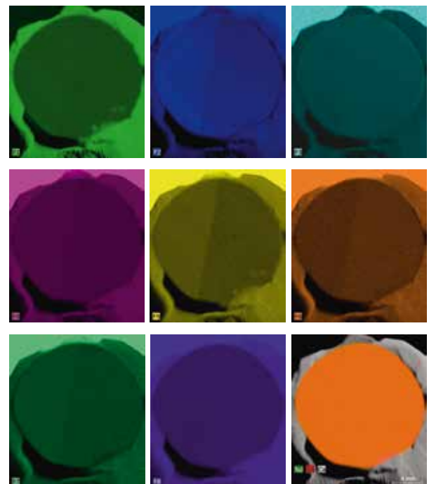
Fig. 4 Color coded crystal domain map and visualization of the Ga and Nd distribution and of the diffractions peaks (F1–F8).
