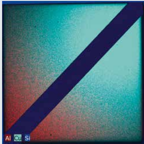
Fig. 3 Elemental distribution of the Cu and Al coated glass substrate
