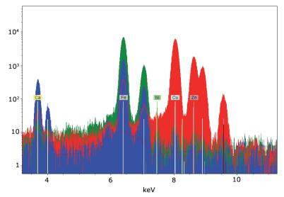
Figure 7 Spectra of the measurement points (MP1: blue, MP2: red, MP3: green)
