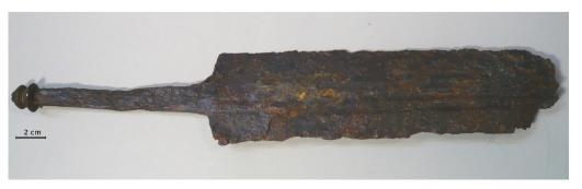
Image of the Roman sword showing the remaining corrosion patina after cleaning.
